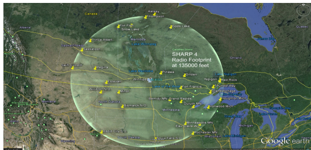
SHARP-4 radio footprint with the balloon near Winnipeg at 135 000 feet
