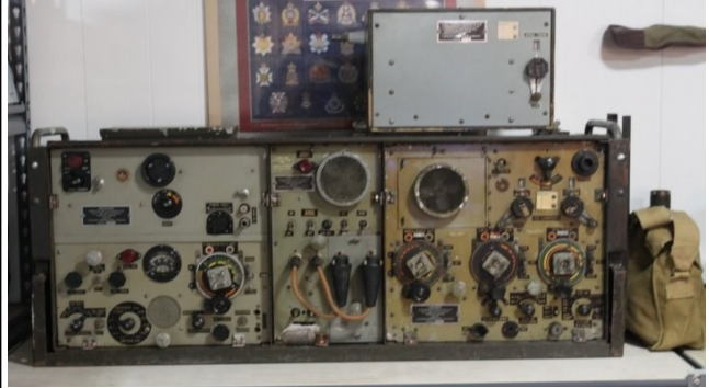
Photo 1: The Main Set Assembly shortly after receiving it from Quebec. Receiver on the left, Supply Unit in the centre and Sender on the right. The Coils, Aerial Tuning No. 2A is on top of the Carriers No. 4.
