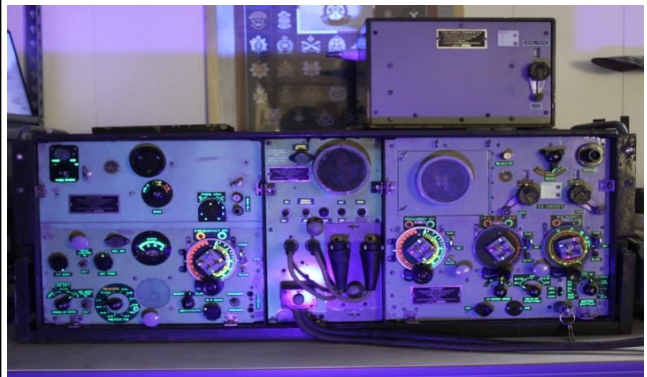
Photo 3: Front view of the Main Set under UV Light showing the luminous markings restored to date.
