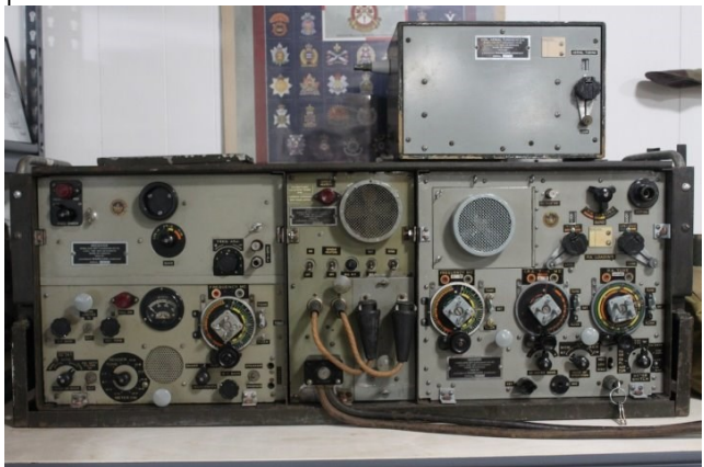
Photo 2: The Main Set after the restoration of the Sender and restoration of the handles and luminous markings on the Receiver.
